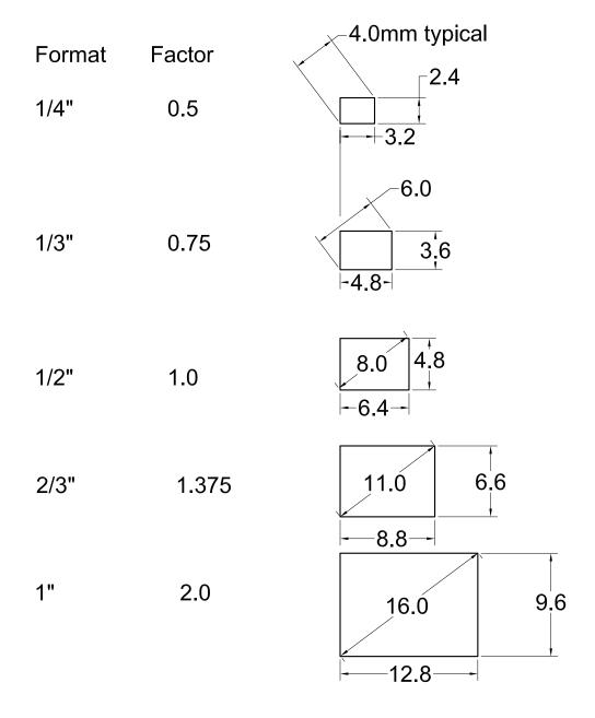
Unless otherwise noted all data is given for 1/2" camera sensors. For FOV or magnification in other sensor sizes use the factors listed. For example, a FOV of 25mm listed for a 1/3" camera would be  $25 \times 0.75 = 18.75$ mm.
