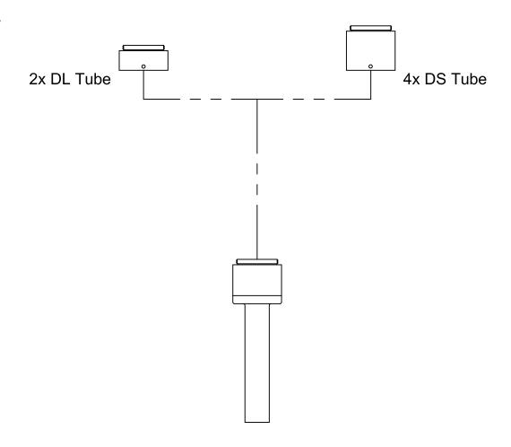
16mm W.D./4x 16mm W.D./8x w/DL Tube 16mm W.D./16x w/DS Tube NA = 0.18
